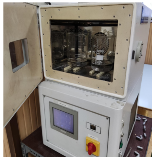
Fig. 2. Corrosion test in climate test chamber
